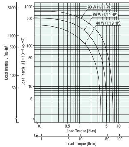
● Speed at Output Shaft: 50 r/min
