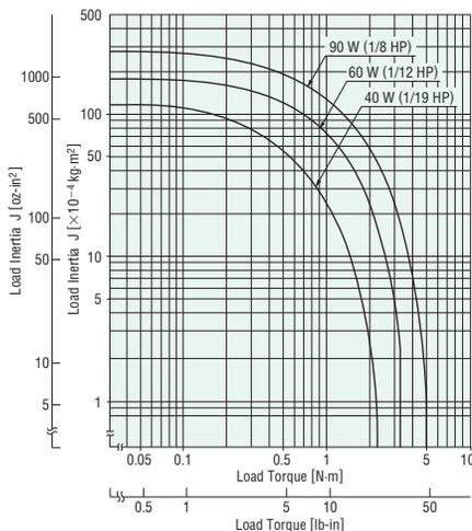
● Speed at Output Shaft: 60 r/min
