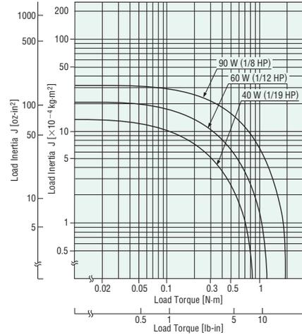
● Speed at Output Shaft: 200 r/min
