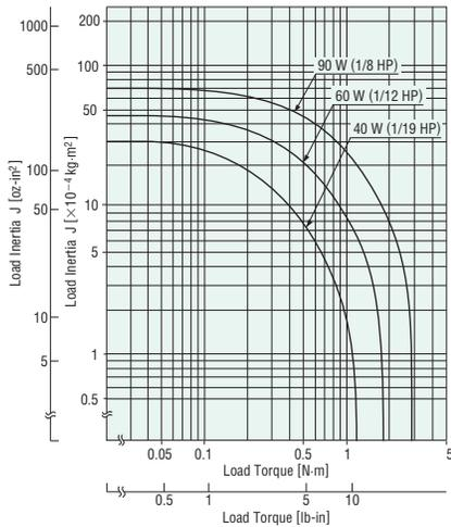
● Speed at Output Shaft: 120 r/min
