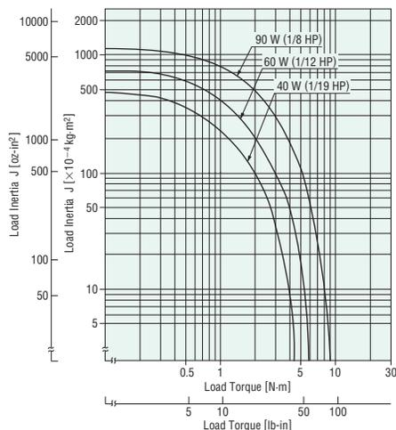
● Speed at Output Shaft: 30 r/min or slower
