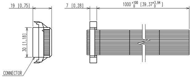
◇ **Motor lead wire / connector assembly**
