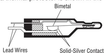
The thermal protectors employ a bimetal contact, using solid silver. Solid silver has the lowest electrical resistance of all materials and has thermal conductivity second only to copper.
