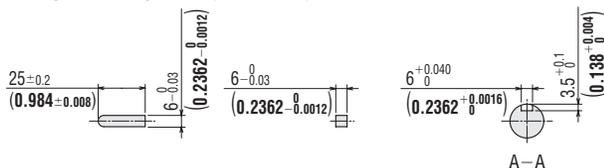
◇ Motor/Hollow Shaft Flat Gearhead
