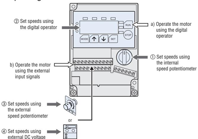
One of the following two operating methods (a and b) can be set by switching between the digital operator mode and external input signal mode.
