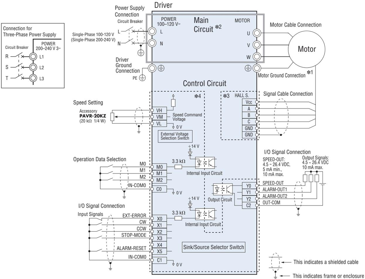
\*1 The grounding method will vary depending on the length of the connection cable.
