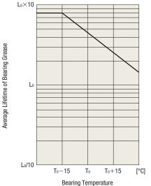
Taking measures to lower the motor temperature is effective for extending the motor's life.
