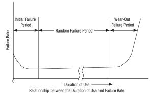
The risks of initial failures are eliminated in the manufacturing and inspection processes, but random failures are sudden failures that occur randomly and unexpectedly during the durable life of the product before wear progresses. Therefore, it is difficult to provide technical measures against random failures, and the only measure available presently is to predict occurrences based on statistical data.
