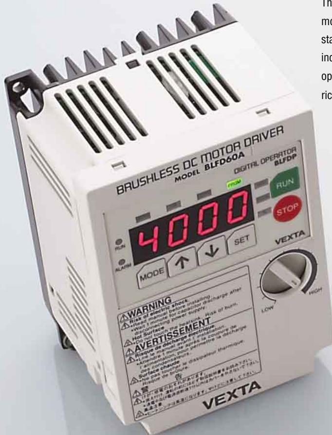
The **BLF** Series combines the attractive features of a brushless DC motor, such as compact size, high output, flat torque, excellent speed stability and energy-saving design, with exciting new enhancements that include a wider speed range and multi-speed operation. Using the digital operator, you can draw the maximum performance out of this feature-rich **BLF** Series with ease.
