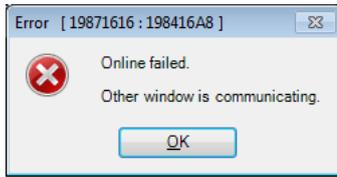
Other data setting window may be executing the communication function. While one window is executing the communication function, other windows cannot use it. Check this point using the following procedure:
