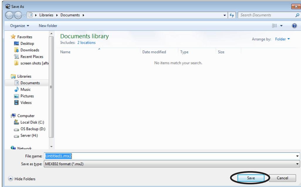
**Note** If the data, which has been saved in the **MEXE02** extended format (.mx2a), will be saved in the **MEXE02** format (.mx2) again, the extended information will be erased. Be sure to check the saving format (filename extension) beforehand.
