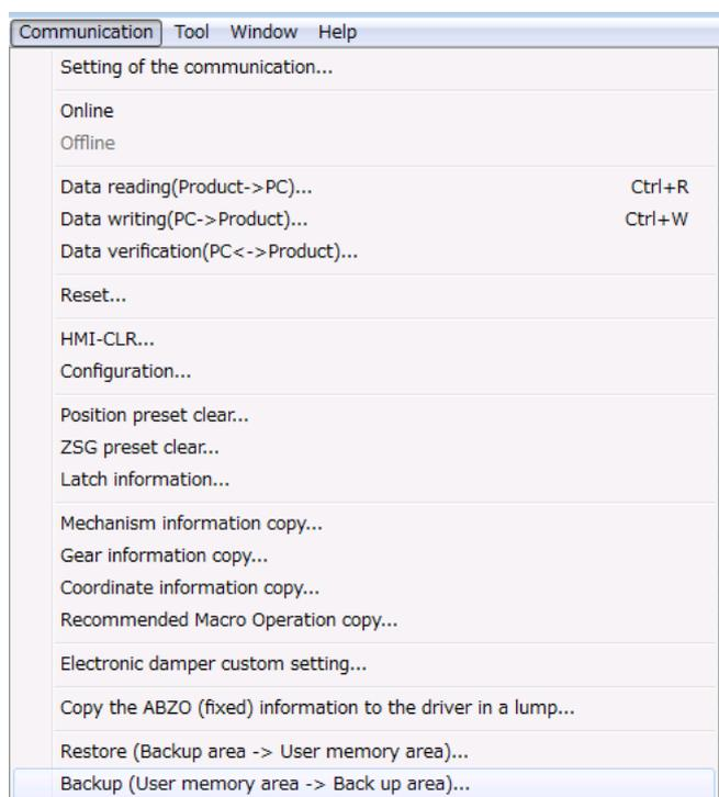
2. Enter the access and write keys (numbers shown under the input field) and click [Backup].
