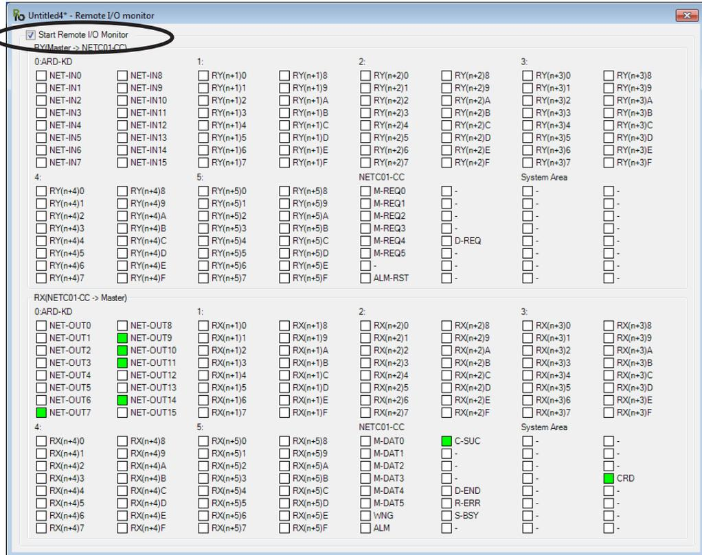
The ON/OFF status of I/O signals is displayed as shown below.
