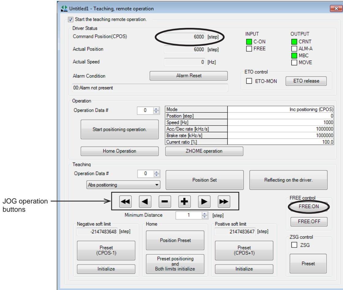
3. Click [Preset (CPOS-1)] to set a software limit value in the negative direction. Click [Preset (CPOS+1)] to set a software limit value in the positive direction.
