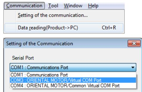
**Note** Before setting the communication port, make sure to connect the PC and applicable product and turn on the power of the applicable product. Without proper connection, the connection port will not be displayed.
