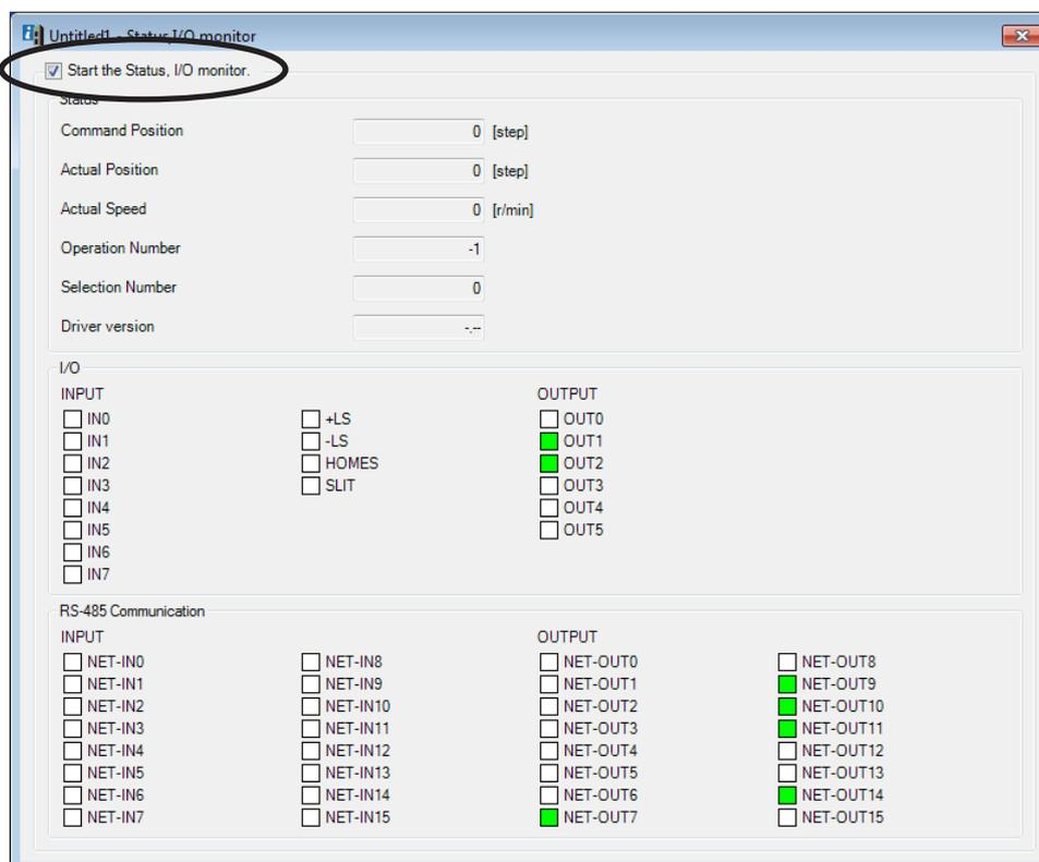
The ON/OFF status of I/O signals is displayed as shown below.
